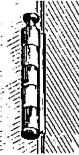
There are hinges which have non-removable pins or hinges containing set screws to prevent pin removal.
