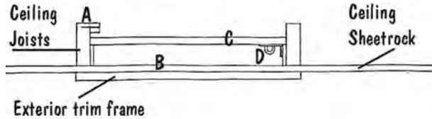
When the crawlway opening is not installed inside the home or storeroom, it should be secured by other means. Secure the crawlway with the following:
