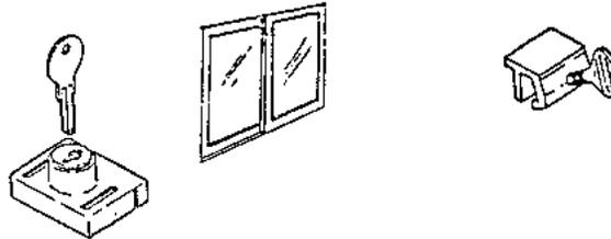
Install wood screws in the upper track above the window. The screw heads should just clear the window, allowing it to slide, but not lift. A wood dowel the appropriate diameter can be used in place of the screws. The dowel should be the same width as the sliding portion of the window.
