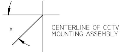
X = THE ROTATION OF THE CCTV CAMERA SHALL BE ALIGNED TO POINT AT THE TRAFFIC SIGNAL POLE ON THE DIAGONALLY OPPOSITE CORNER, UNLESS OTHERWISE INSTRUCTED BY THE CITY.
